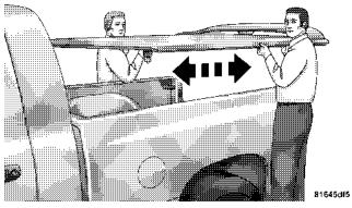
Carrying Cover Toward The Rear Of the Vehicle Reverse the procedure for installation.
